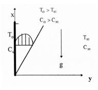
Figure 1 Flow near the plate
