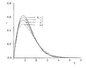
Figure 8 The variation of the dimensionless velocity  $\phi'$  with  $\beta_2$  for Pr = 0.73, Sc = 1.4, N = 3,  $\beta_1 = 4.0$ ,  $\alpha = -0.4$ ,  $\beta_2 = 0, 1, 2, 3$
