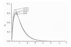
Figure 2 The variation of the dimensionless velocity  $\phi'$  with  $\alpha$  for Pr = 0.73, Sc = 1.4, N = 3,  $\beta_1 = 4.0$ ,  $\beta_2 = 3.0$ ,  $\alpha = -0.1$ , -0.2, -0.3, 0.4
