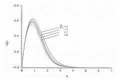
Figure 3 The variation of the dimensionless velocity  $\phi'$  with  $\alpha$  for Pr = 4, Sc = 10, N = 3,  $\beta_1 = 0.12$ ,  $\beta_2 = 0.1$ ,  $\alpha = 0, 0.1, 0.2, 0.6$
