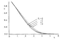
Figure 9 The variation of the dimensionless temperature  $\theta$  with  $\beta_2$  for Pr = 0.73, Sc = 1.4, N = 3,  $\beta_1 = 4.0$ ,  $\alpha = -0.4$ ,  $\beta_2 = 0, 1, 2, 3$
