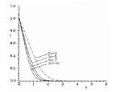
Figure 18 The variation of the dimensionless concentration  $\gamma$  with Sc for N = 3, Pr = 4,  $\beta_1 = 0.12$ ,  $\beta_2 = 0.1$ ,  $\alpha = 0.6$ , Sc = 2, 5, 7, 10
