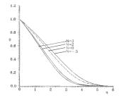
Figure 12 The variation of the dimensionless temperature  $\theta$  with N for Pr = 0.73, Sc = 1.4,  $\alpha = -0.4$ ,  $\beta_2 = 3.0$ , N = -0.5, 0, 1, 2, 3
