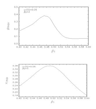
Figure 3 Amplitudes of the pendulum versus frequency ratio  $\beta_1$  (internal resonant curves) for  $y_1(0) = 0.05$  and d = 0.02,  $\beta_2 = 2$ ,  $\gamma_1 = \gamma_2 = 0$ , q = 0
