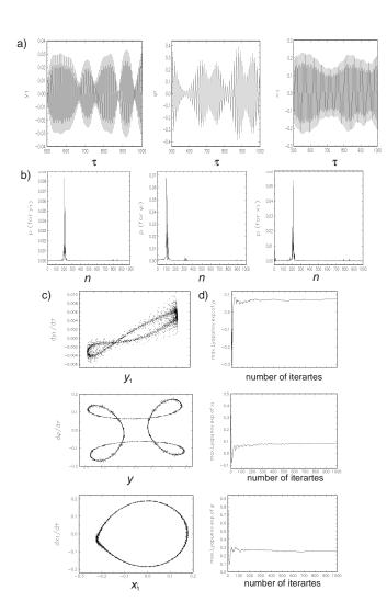
**Figure 6** Time history (a) , power spectral density (FFT) (b), Poincaré map (c) and maximum Lyapunov exponent(d) corresponding to coordinates  $y_1$ ,  $x_1$  and  $\varphi$  for:  $\beta_1 = 0.5$ ,  $\beta_2 = 2$ , d = 0.02,  $\gamma_1 = 0$ ,  $\gamma_2 = 0.0002$ , q = 0.0005,  $\mu = 1.07$
