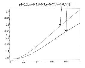
Figure 2 The dimensionless growth rate x as a function of dimensionless wave number r to show the effect of magnetic field
