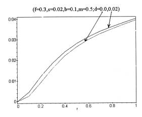
**Figure 3** The dimensionless growth rate x as a function of dimensionless wave number r to show the effect of porous media
