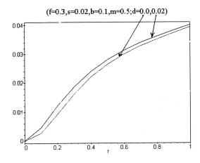
Figure 4 The dimensionless growth rate x as a function of dimensionless wave number r to show the effect of heat transfer
