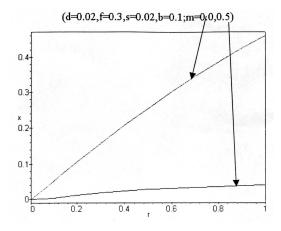
Figure 5 The dimensionless growth rate x as a function of dimensionless wave number r to show the effect of surface tension
