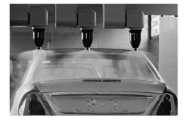
${\bf Figure \ 14} \ {\rm The \ process \ of \ nanolaquer \ application \ in \ the \ factory \ of \ Mercedes-Benz$
