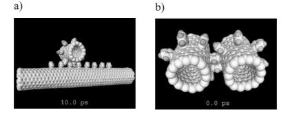
Figure 6 Nano-gear created from individual atoms
