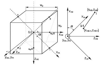
Figure 8 Transformations of dimensions between local systems of reference
