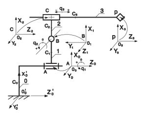
Figure 5 Kinematic scheme of the NM7MAR manipulator. Selection of systems of co-ordinates of links
