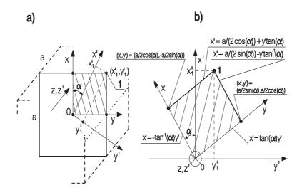
${\bf Figure \ 10} \ {\rm Scheme \ of \ transformations \ of \ geometrical \ dimensions \ in \ local \ systems}$
