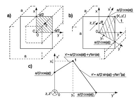
Figure 9 Scheme of transformations of geometrical dimensions in local systems of reference
