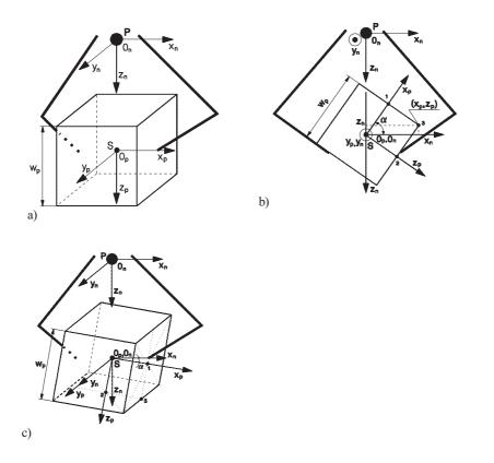
**Figure 4** The manipulator gripping device - manipulated object system. Exemplary selection of local systems of reference for the case of the object manipulated in the form of a homogeneous cube: a) matrix of transformation of local systems of reference according to Eq. (19); b), c) matrix of transformation of local systems of reference according to Eq. (30). The local system of reference of the manipulated object  $(x_p y_p z_p 0_p)$  is its main central system of inertia
