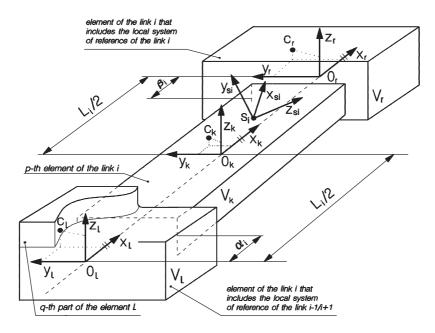
Figure 1 Structural division of the *i*-th link of the manipulator
