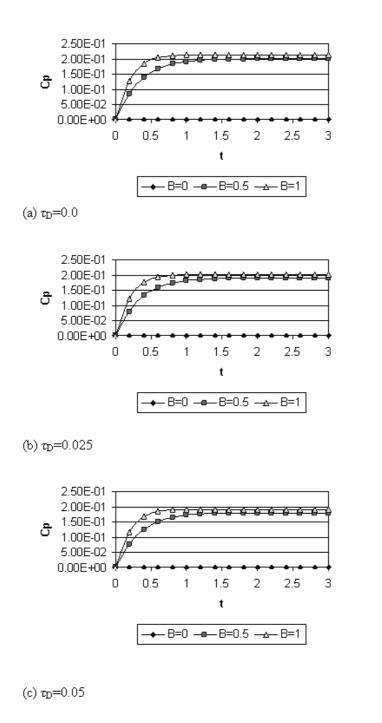
Figure 10 Time development of  $C_p$  for various values of  $\tau_D$  and  $\beta$
