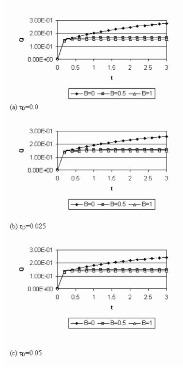
Figure 7 Time development of Q for various values of  $\tau_D$  and  $\beta$
