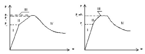
Figure 1 Load paths of thin–walled beam–column, a) – elastic buckling of the weakest plate element, b) – elasto–plastic buckling of the weakest plate element
