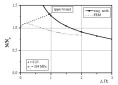
Figure 9 Loading path of rectangular steel plate of dimension  $1600 \times 800 \times 50$  [mm], (pitched roof mechanism for energy method – s = 0.25)
