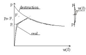
Figure 2 Thin–walled column subject to eccentric compression. Lower and upper bound estimation of the load–capacity
