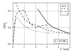
Figure 10 Load-deflection diagrams for steel channel section column: 1 - energy method, 2 - equilibrium strip method, 3 - experimental results [9], 4 - FE results, height of the web = 102 mm, width of the flange = 38.33 mm, wall thickness = 1 mm
