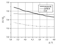
Figure 8 Failure curves of rectangular steel plate of dimension  $1600 \times 800 \times 50$  [mm]
