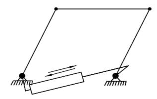
Figure 2 Four bar linkage modeling landing gear
