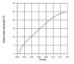
Figure 10 Rotation angle velocity of the crank versus time with (----) and without ( ----) friction
