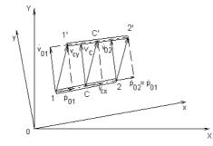
Figure 5 Displacement of a rigid finite element in global and local coordinates
