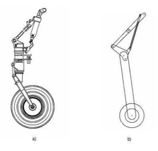
Figure 1 Constructional model of landing gear (a) and its beam-type model (b)
