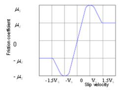
Figure 8 Change of friction coefficient with slip velocity
