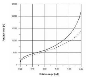
Figure 12 Minimal actuator force needed for gear rotation with (--) and without (---) friction forces versus rotation angle
