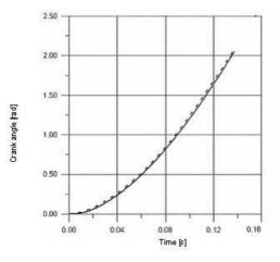
Figure 6 Crank angle versus time for FEM model (----) and ADAMS model (-----)
