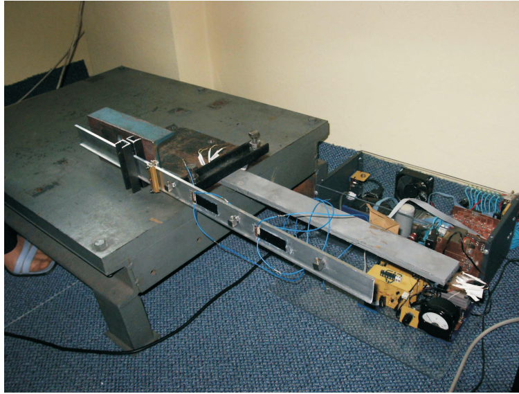
Figure 2 Test stand configuration with piezoelectric sensor / actuator
