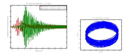
a) Components of vibration amplitude along x,y axes and 2D motion trajectory of centroid
