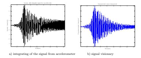
**Figure 5** Value component of the vertical movement along the y-axis derived from the system of video (b) and integration of signal from accelerometer (a) a) integrating the signal from accelerometer b) the differential video signal
