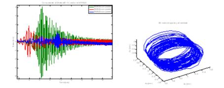
b) Components of vibration amplitude along x,y,z axes and 3D motion trajectory of centroid
