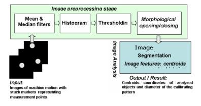
Figure 1 Diagram used in the transition falling developed an algorithm for image analysis
