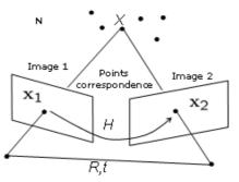
Figure 2 Homography matrix describing the relationship between the projections of points lying on one plane of the normal vector N on the plane imaging cameras 1 and 2
