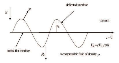
Figure 1 Sketch of a gravitating compressible fluid layer under the effect of the capillary pressure and a horizontal magnetic field
