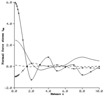
Figure 2 Variation of Normal force stress  $t_{22}$  with horizontal distance x due to concentrated force
