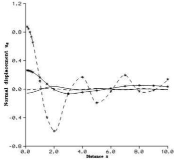
Figure 4 Variation of Normal displacement  $u_2$  with horizontal distance x due to uniformly distributed force
