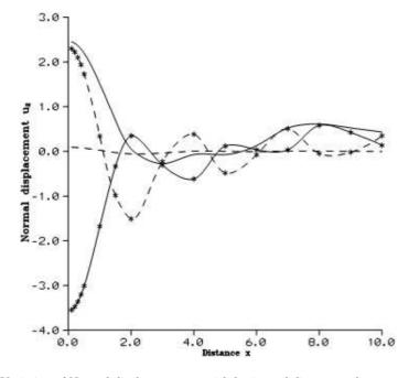
Figure 7 Variation of Normal displacement  $u_2$  with horizontal distance x due to a moving force 5.0  $\neg$
