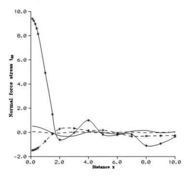
Figure 5 Variation of Normal force stress  $t_{22}$  with horizontal distance x due to uniformly distributed force
