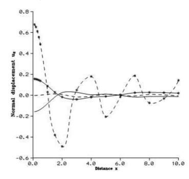
Figure 1 Variation of Normal displacement  $u_2$  with horizontal distance x due to concentrated force
