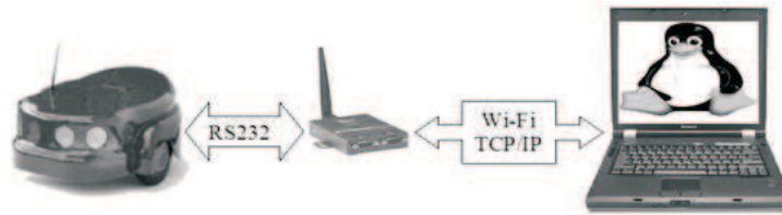
Figure 5 Elements of the mechanism of communication robot – computer
