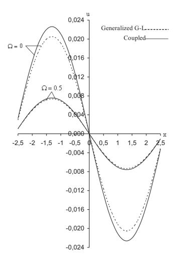
Figure 8 Horizontal displacement distribution **u** on the middle plane at t = 0.1.
