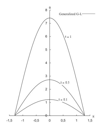
Figure 7 Temperature distribution  $\theta$  on the middle plane at  $\Omega = 0$  and 0.5.
