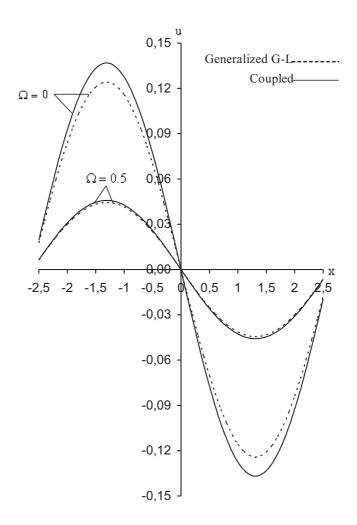
Figure 9 Horizontal displacement distribution **u** on the middle plane at t = 1.
