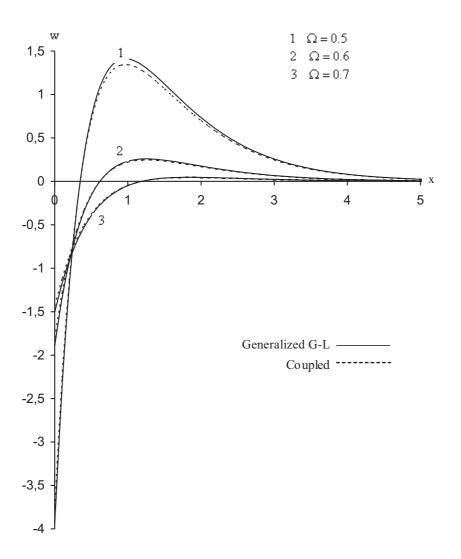
Figure 9 Distribution of displacement component w for z=0 and  $\alpha=1.02$
