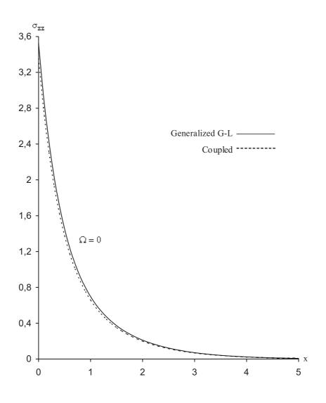
Figure 5 Distribution of stress component  $\sigma_{zz}$  for z = 0 and  $\Omega = 0$
