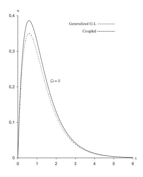
Figure 2 Distribution of displacement component u for z=0 and  $\Omega=0$
