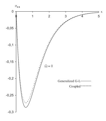
Figure 6 Distribution of stress component  $\sigma_{xz}$  for z = 0 and  $\Omega = 0$
