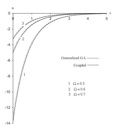
Figure 8 Distribution of displacement component u for z=0 and  $\alpha=1.02$
