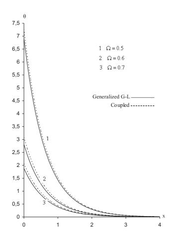
Figure 7 Temperature distribution for z=0 and  $\alpha=1.02$
