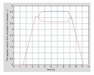
Figure 3 The angular velocities time courses from simulation:  $\dot{\alpha_1}$  [rad/s]– blue,  $\dot{\alpha_2}$  [rad/s]– red
