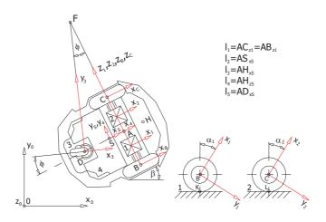
Figure 1 Computation model of  $\operatorname{AmigoBot}^{TM}$  robot
