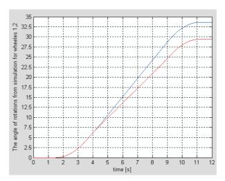
Figure 2 The angles of rotations time courses from simulation:  $\alpha_1$  [rad] – blue,  $\alpha_2$  [rad] – red
