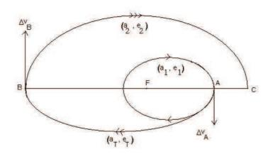
Figure 4 Apogee of transfer orbit coincides with apogee of final orbit. (Initial impulse at apogee)
