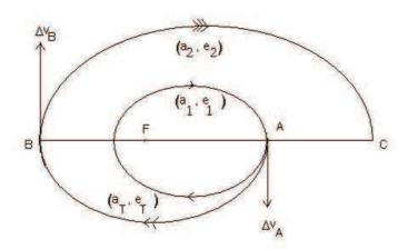
$\textbf{Figure 3} \ \text{Perigee of transfer orbit coincides with perigee of final orbit.} \ (\text{Initial impulse at apogee})$
