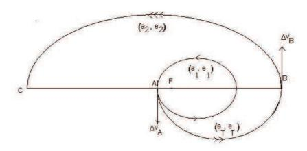
Figure 2 Apogee of transfer orbit coincides with perigee of final orbit. (Initial impulse at perigee)
