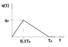
Figure 2 Pressure pulse shape: q(t) – pressure,  $T_p$  – duration of the pulse,  $q_a$  – amplitude of pressure the pulse
