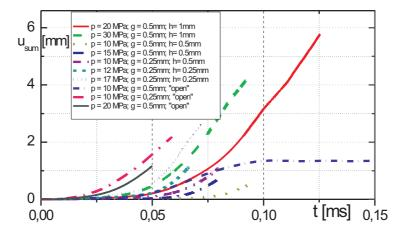
Figure 6 Curves of the maximal summary displacement in the whole structure versus time for different pressure amplitudes
