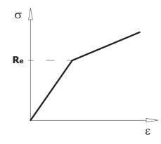
Figure 3 Bilinear strain-stress curve of the ultimate strength:  $R_e$  - yield stress
