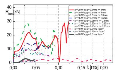
Figure 7 Curves of the ground reaction versus time for different pressure amplitudes
