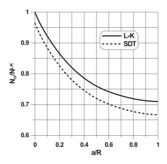
Figure 2 Influence of width of piezoelectric layer on value of critical force (L–K – Love-Kirchhoff theory, SDT – first order shear deformation theory)
