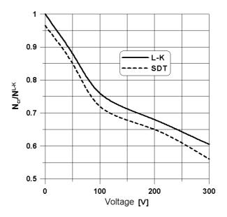
Figure 3 Influence of voltage on value of critical force (L–K – Love–Kirchhoff theory, SDT – first order shear deformation theory)
