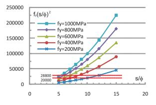
**Figure 5** Graphs of relations  $f_y (s/\phi)^2$  for various yield strengthes
