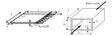
Figure 1 Simply supported plate and thin-walled column (A - cross-section area)
