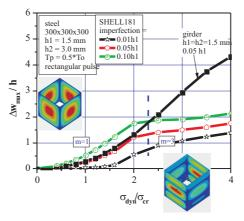
Figure 6 Influence of imperfections and different wall thickness on column dynamic response
