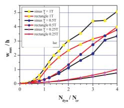
Figure 4 Influence of pulse shape and duration on plate dynamic response (geometric parameters the same as in Fig.3)
