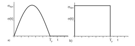
Figure 2 Exemplary shapes of pulse loading a) sinusoidal b) rectangular
