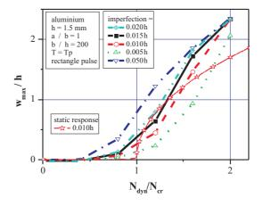
Figure 3 Influence of initial deflection amplitude on plate dynamic response
