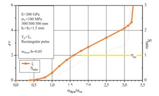
Figure 8 Dimensionless maximal dynamic deflection  $\xi = \Delta w_{max}/h$  and effective stress ratio for cubic column (material characteristic)
