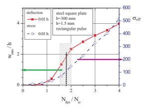
Figure 10 Comparison of dynamic buckling load estimated on the basis of three buckling criteria
