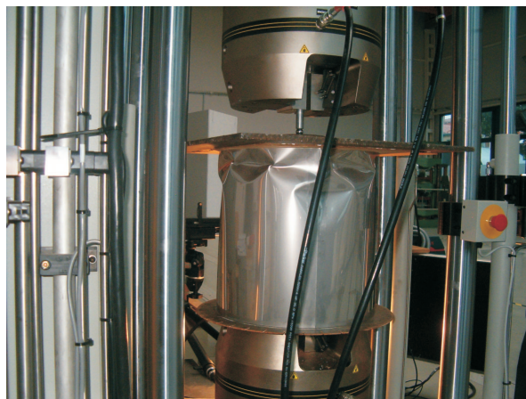
Figure 5 The test rig. The collapse of the tested cylinder
