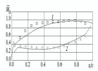
Figure 3 The Mach number (b) distribution over the blade chord (1 suction side, 2 pressure side, [][] pressure side experiment,  $\times \times$  suction side experiment)
