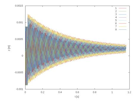
Figure 6 Bending blade motion with 150 Hz excitation frequency and +45 deg phase angle in long time response
