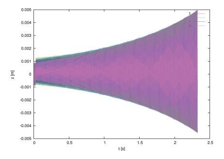
Figure 5 Bending blade motion for 150 Hz excitation frequency and -90 deg phase angle in long time response
