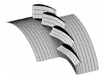
Figure 1 A view of a sector of the whole blade assembly
