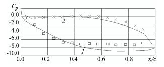
Figure 2 The time averaged pressure coefficient distribution over the blade chord (1 suction side, 2 pressure side, [][] pressure side experiment,  $\times \times$  suction side experiment)
