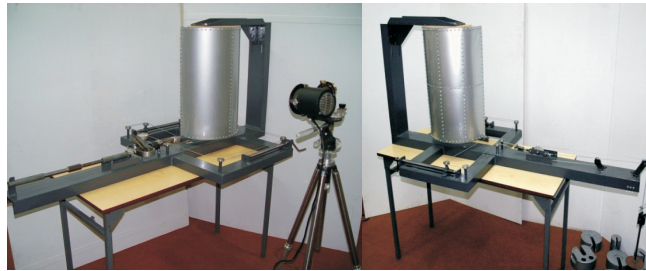
Figure 1 A stand for testing thin-shell structures subject to torsion: left – a version with a loading system controlling the displacement (turnbuckle), right – a version with a system controlling by force (gravitational)
