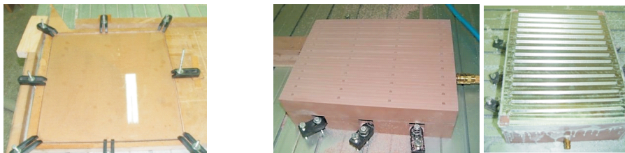
Figure 6 Mounting methodes and vacuum table used in manufacturing process
