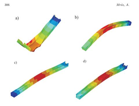
Figure 6 Dynamic response to impulse compression pressure of the profile with cross section: a) C channel, b) Rectangular, c) Internal tandem, d) External tandem
