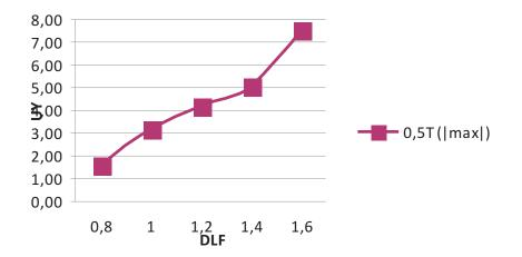
Figure 8 Dynamic deflection obtained with the FEM for Internal tandem- time duration of compression impulse equals  $0.5 \times natural period$  (of 1st mode)
