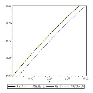
Figure 2 Effect of Reynolds number on axial velocity
