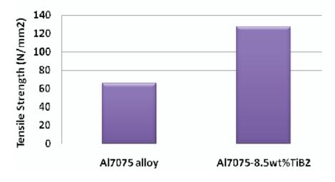
Figure 4 Tensile Strength of Al7075 alloy and Al7075-TiB<sub>2</sub>composite
