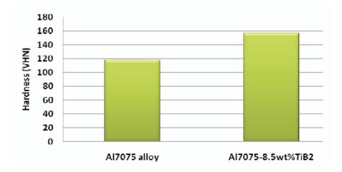
Figure 3 Hardness of Al7075 alloy and Al7075-TiB<sub>2</sub> copmpsite
