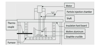
Figure 1 Stir casting Experimental set up
