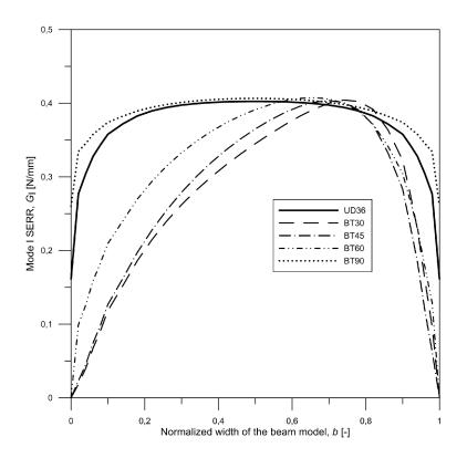
Figure 1 Mode I SERR variability along the width of the B-T coupled laminate beam model
