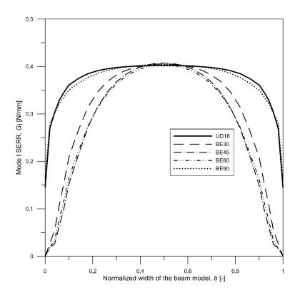
Figure 2 Mode I SERR variability along the width of the B-E coupled laminate beam model
