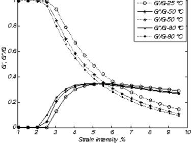
Figure 10 The real and imaginary parts of complex modulus at various temperatures
