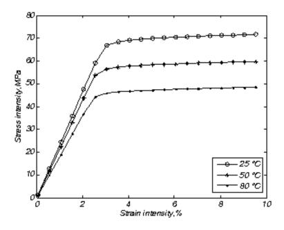
Figure 9 Cyclic diagram for 1 Hz at 25, 50 and  $80^{\circ}$ C
