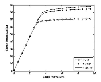
Figure 7 Cyclic diagram for PR-520 at 1, 50 and 100 Hz  $\,$
