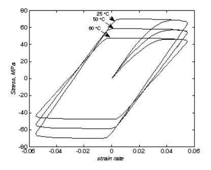
Figure 4 Actual loops under cyclic loading
