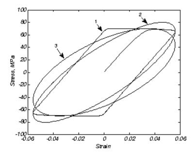
Figure 6 Hysteresis loops at the frequency 1 Hz  $\,$
