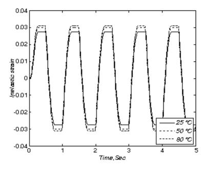
${\bf Figure}~{\bf 3}$  Inelastic strain evolution under kinematic harmonic loading
