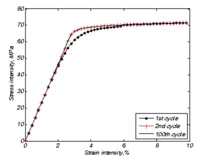
Figure 5 Stabilized cyclic diagram for PR–520 at 1 Hz  $\,$
