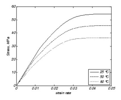
Figure 1 The stress–strain curve under monotonic loading in pure shear
