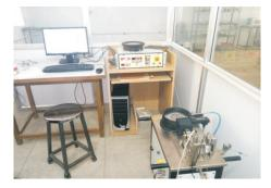
Figure 2 Pin on disc wear test rig
