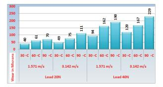
Figure 3 Effect of temperature, load and sliding velocity on wear of AA 7075 - SiC composite
