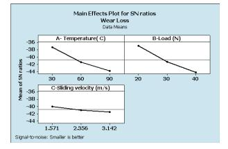
Figure 5 The main effects plot for S/N ratio
