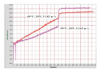
Figure 4 Effect of temperature on wear of AA 7075 - SiC composite
