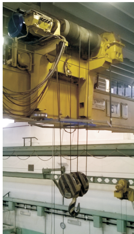
Figure 10 Rope system of the crane with measuring systems
