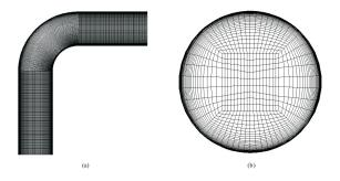
Figure 2 Computational grid of the geometry
