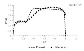
Figure 3 Comparison between Normalized axial velocity profiles of present analysis with published experimental results
