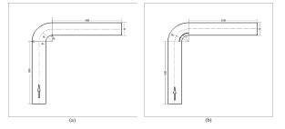
Figure 1 Schematic Diagram of the bend geometry: a) Without guide vane, b) With guide vane
