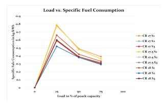
Figure 2 Response values of Specific Fuel Consumption at various loads for each sample
