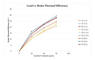
Figure 3 Response values of Brake Thermal Efficiency at various loads for each sample
