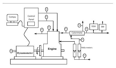
Figure 1 Layout of the engine set up
