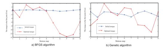
${\bf Figure}~{\bf 5}$  The torque in the first joint before and after optimization
