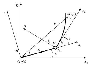
Figure 1 The schematic diagram of a two-link rigid-flexible manipulator
