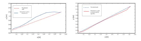
Figure 4 Comparison between the traveled path by the manipulator and the desired path using the BFGS and the genetic algorithms
