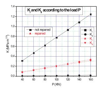
Figure 5 Propagation of cracks in notched beam before and after reparation
