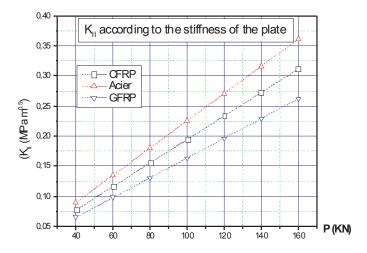
Figure 11 Stress Intensity factor  $K_{II}$  in repaired beam based on the stiffness of the plate (where Lp = 2400 mm, thickness t = 4 mm)
