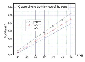
Figure 9 Stress Intensity factor  $K_{II}$  in repaired beams according to the thickness of the plate for a length of strengthening Lp = 2400 mm
