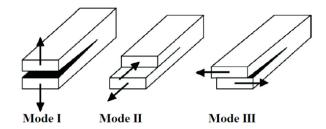
Figure 2 Three basic modes of fracture propagation
