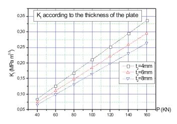
Figure 6 Stress Intensity factor  $K_I$  in repaired beams according to the thickness of the plate for a length of strengthening Lp = 2400 mm
