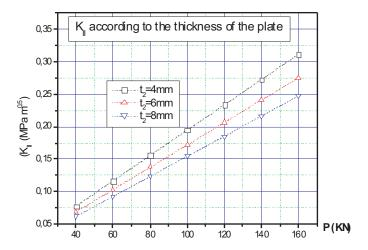
Figure 7 Stress Intensity factor  $K_I$  in repaired beams based on the stiffness of the plate for a length plate Lp = 2400 mm, thickness = 4 mm
