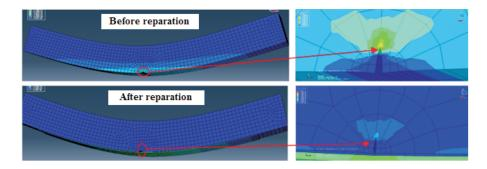
${\bf Figure}~4$  Effect of CFRP on the behaviour of cracked beams
