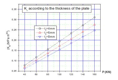
Figure 10 Stress Intensity factor  $K_{II}$  in repaired beams based on the stiffness of the plate for a length plate Lp = 2400 mm, thickness = 4 mm
