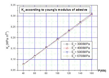
Figure 8 Stress Intensity factor  $K_I$  in repaired beams based on the stiffness of the plate for a length plate Lp = 2400 mm, thickness = 4 mm
