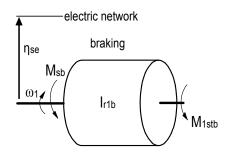
Figure 2 A physical model of electric braking of the system of an overhead crane travelling
