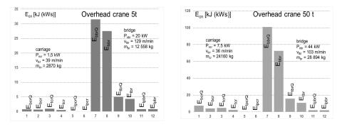
Figure 4 Distribution components of the energy profits in a norm cycle of overhead cranes
