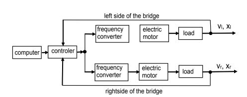
Figure 3 A scheme of supplying and controlling motors of end-carriages of an overhead crane bridge
