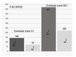
Figure 6 Energy profits  $E_{cn}$  in a norm cycle in comparison to the energy use  $E^*_{cn}$  of the drives without frequency convertors
