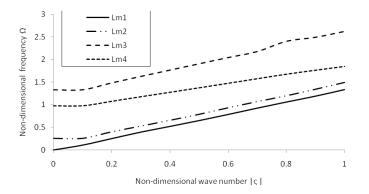
Figure 2 Non-dimensional wave number  $|\varsigma|$  versus Non-dimensional frequency  $\Omega$  of longitudinal modes of vibration for a piezoelectric cylindrical fiber without coating
