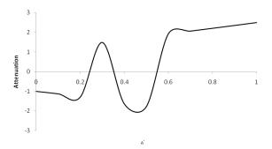
Figure 7 Variation of Attenuation versus thickness of the coating material  $h^{'}$  for real part longitudinal mode
