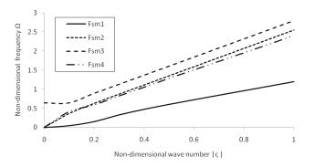
**Figure 4** Non-dimensional wave number  $|\varsigma|$  versus Non-dimensional frequency  $\Omega$  of flexural symmetric modes of vibration for a piezoelectric cylindrical fiber without coating
