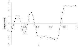
Figure 9 Variation of Attenuation versus thickness of the coating material  $h^{'}$  for real part of flexural anti symmetric mode
