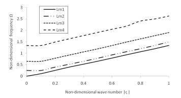
Figure 1 Non-dimensional wave number  $|\varsigma|$  versus Non-dimensional frequency  $\Omega$  of longitudinal modes of vibration for a piezoelectric cylindrical fiber with coating
