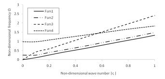
Figure 3 Non-dimensional wave number  $|\varsigma|$  versus Non-dimensional frequency  $\Omega$  of flexural symmetric modes of vibration for a piezoelectric cylindrical fiber with coating
