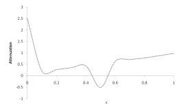
Figure 12 Variation of Attenuation versus thickness of the coating material h' for imaginary part of flexural symmetric mode
