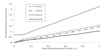
**Figure 5** Non-dimensional wave number  $|\varsigma|$  versus Non-dimensional frequency  $\Omega$  of flexural antisymmetric modes of vibration for a piezoelectric cylindrical fiber with coating
