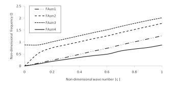
Figure 6 Non-dimensional wave number  $|\varsigma|$  versus Non-dimensional frequency  $\Omega$  of flexural antisymmetric modes of vibration for a piezoelectric cylindrical fiber without coating
