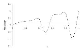
Figure 11 Variation of Attenuation versus thickness of the coating material  $h^{'}$  for real part of flexural symmetric mode
