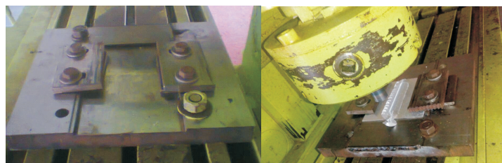
Figure 6 Complete Fixture Base plate, with clamp and stopper fitted on machine table
