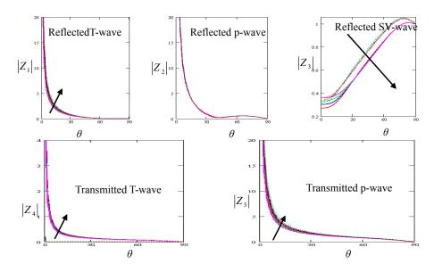
Figure 10 Variation of the amplitudes  $z_i$  (i = 1, 2, ..., 5) with the angle of incidence of SV-wave for variation of initial stress:  $P = (1.1, 1.2, 1.3, 1.4) (10)^{11}$ , H = 0.3 (—), H = 0 (...)
