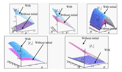
Figure 8 Variation of the amplitudes  $z_i$  (i = 1, 2,..., 5) with respect to  $(\theta, H)$  of thermal-wave with and without variation of initial stress
