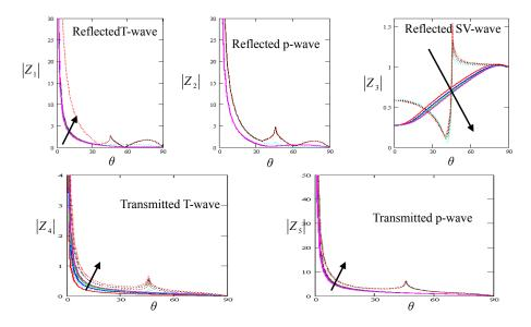
**Figure 9** Variation of the amplitudes  $z_i$  (i = 1, 2,..., 5) with the angle of incidence of SV-wave for variation of magnetic field: H = 0.1, 0.2, 0.3, 0.4, P =  $1.1(10)^{11}$  (—), P = 0 (...)
