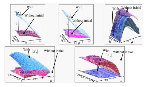
Figure 5 Variation of the amplitudes  $z_i$  (i = 1, 2, 5) with respect to of p-wave with and without variation of initial stress
