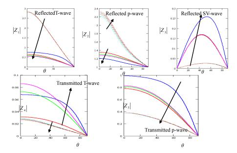
Figure 4 Variation of the amplitudes zi (i = 1, 2,, 5) with the angle of incidence of p-wave for variation of initial stress:  $P = (1.1, 1.2, 1.3, 1.4) (10)^{11}$ , H = 0.3 (—), H = 0 (...).
