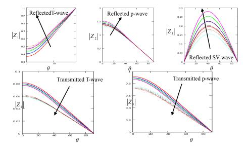
Figure 7 Variation of the amplitudes  $z_i$  (i = 1, 2, ..., 5) with the angle of incidence of thermal-wave for variation of initial stress: P = (1.1, 1.2, 1.3, 1.4) (10)<sup>11</sup>, H = 0.3 (--), H = 0 (...)
