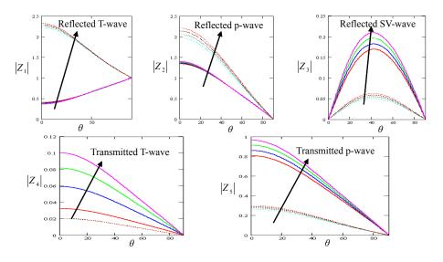
**Figure 6** Variation of the amplitudes  $z_i$  (i = 1, 2, ..., 5) with the angle of incidence of thermal-wave for variation of magnetic field: H = 0.1, 0.2, 0.3, 0.4, P =  $1.1(10)^{11}$  (—), P = 0 (...)
