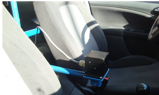
Figure 8 Experimental setup; Crossbow IMU-300CC - Seat Toledo III
