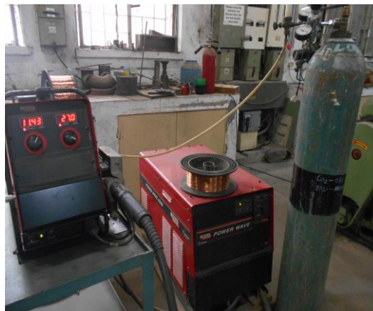
Figure 2 The actual set up of metal inert gas welding (MIG)
