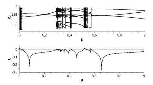
Figure 2 Bifurcation diagram and the LLE graph of the forced van der Pol system (10)
