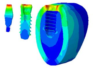
Figure 5 Distribution of the induced Von Mises equivalent stress in the dental structure
