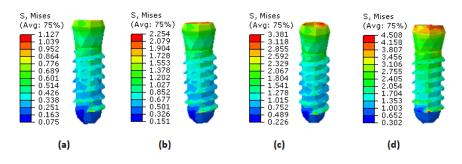
Figure 6 Level and distribution of the equivalent stress of Von Mises induced in the implant
