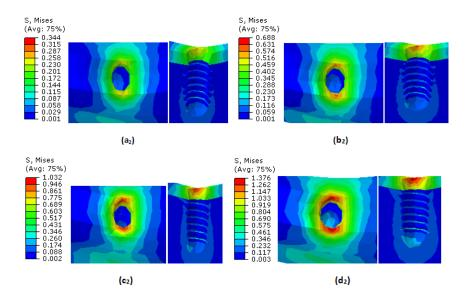
Figure 8 Level and distribution of induced equivalent stress in bone
