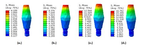
Figure 7 Level and distribution of the equivalent stress of Von Mises induced in the abutment
