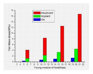
Figure 10 Von Mises stress comparison histograms for each component of the dental structure
