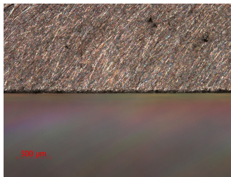
Figure 11 The appearance of edge 3b after brushing, edge fillet 0,117 mm, zoom \times 40
