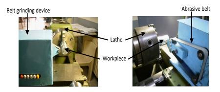
Figure 1 Belt grinding device mounted on a conventional lathe
