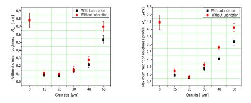
Figure 8 Variation of the surface roughness  $R_a$  and  $R_z$  with respect to the abrasive grains size
