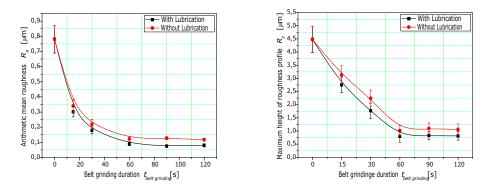
Figure 4 Variation of arithmetic mean roughness  $R_a$  and maximum height of roughness profile  $R_z$  depending on the belt grinding time with and without lubrication
