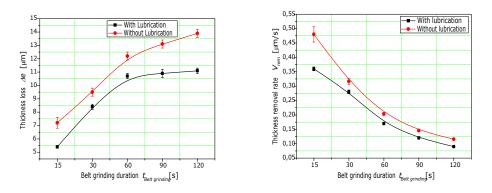
Figure 3 Loss in thickness and thickness removal rate depending on the belt grinding time with and without lubrication
