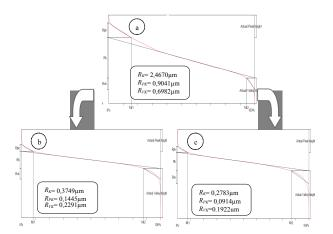
**Figure 7** Evolution of the profile bearing ratio: a) Before belt grinding, b) After belt grinding dry, c) After belt grinding with lubrication, (Conditions:  $t_{beltgrinding} = 60$  s,  $\emptyset = 20 \ \mu m$ , N = 900 rev/min)
