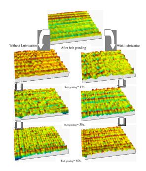
Figure 6 Surface topography according belt grinding time with and without lubrication
