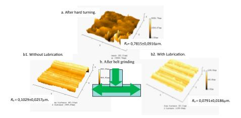
Figure 9 Microscopic image by AFM before and after belt finishing by size  $20\mu m$
