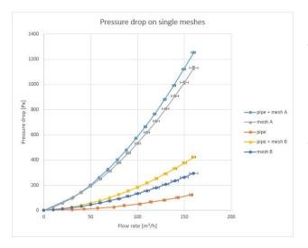
Figure 5: Characteristic of pressure drop vs. flow rate for meshes A and B
