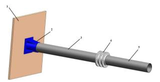
**Figure 2:** Assembly of test piece; 1-adapter plate; 2-adapter; 3-pipe 600 mm; 4-filtration setup; 5-pipe 400 mm
