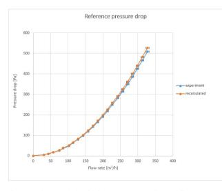
Figure 4: Characteristic of reference pressure drop vs. flow rate
