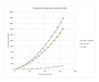
Figure 6: Characteristic of pressure drop vs. flow rate for meshes A+B
