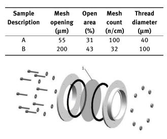
Figure 3: Assembly of Filter setup - single layer; 1-mesh sample
