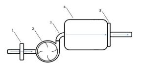
**Figure 1:** Schematic of air performance test rig; 1- measuring section; 2-support fan; 3-connection tube; 4-test chamber; 5-test piece
