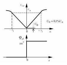
Fig. 1.2. Dependence of the amplitude and phase of the differential transformer sensor on the core displacement
