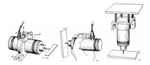
Fig. 1.11. Examples of applications of the electro-dynamic sensor of relative vibrations
