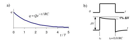
Fig. 1.16. a) discharge curve, b) response to the rectangular excitation
