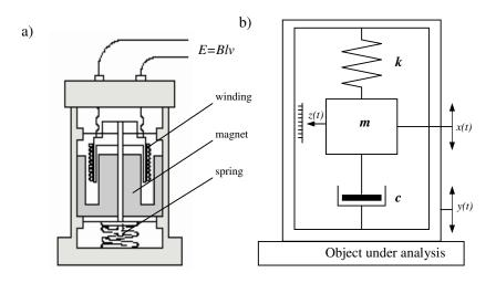
Fig. 1.6. Design and model of the mechanical system of the seismic electro-dynamic sensor
