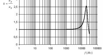
Fig. 1.15. Characteristic curve of the piezoelectric sensor
