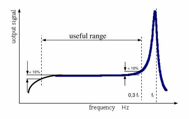
Fig. 1.17. Piezoelectric sensor charcteristic
