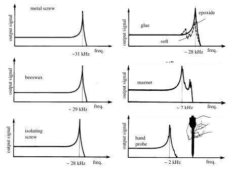
Fig. 1.22. Influence of the sensor fixing type on the resonance frequency
