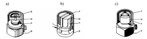
Fig. 1.21. Shear<sup>®</sup> type sensors: a) – traditional shear type, b) – Planar Shear type, c) – Delta Shear<sup>®</sup> type; S – spring, M – seismic mass, P – piezoelectric element, B – base, R – compressing ring
