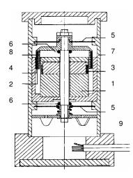
Fig. 1.9. Seismic electro-dynamic sensor, type PR9266: 1 permanent magnet, 2 measurement coil winding, 3 \_ damping winding, correction winding, 5 - membrane spring, 6 - stop, 7 - housing, 8 - shielding cable
