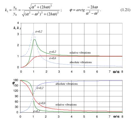
Fig. 1.7. Frequency, amplitude and phase characteristics of the seismic sensor
