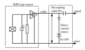
Fig. 1.20. Example of the slotted section of the sensor with integrated electronics
