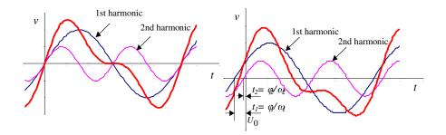
Fig. 1.8. Influence of the phase shift in the electro-dynamic sensor on non-linear deformations
