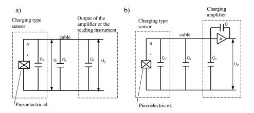
Fig. 1.18. Scheme of the system: a) with a voltage amplifier, b) with a charge amplifier
