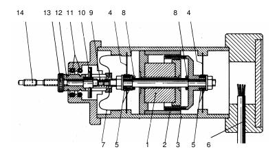
Fig. 1.10. Electro-dynamic sensor, type PR9267 (Philips):
