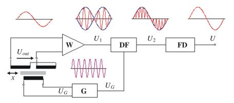
Fig. 1.4. Block scheme of the sensor with phase-sensitive rectification
