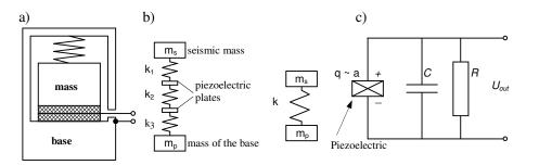
Fig. 1.14. Piezoelectric acceleration sensor: a) scheme, b) equivalent mechanical model, c) equivalent electrical model
