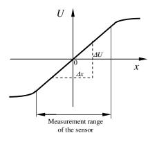
Fig. 1.5. Static characteristic of the system with phase-sensitive rectification
